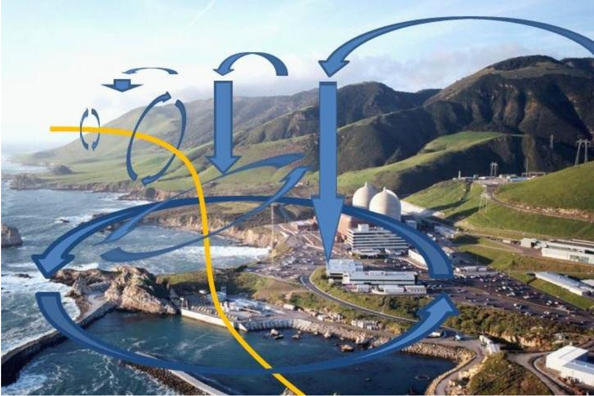
755 Figure 11. Schematic depiction of the “backwards” rolling horizontal vortex tube being 756 tilted downward into a vertical orientation by the differential vertical velocities between 757 the weak or nonexistent downward motion on the periphery of the high terrain and the 758 maximum downward motion at the terrain centerline (see Figure 3c in Rotunno and 759 Smolarkiewicz 1991) . Viewing upwind against the flow as in this figure, this produces a 760 cyclonically rotating vortex to the left of the centerline.
