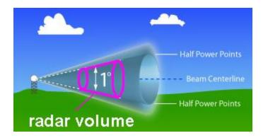
What does this mean? To illustrate, consider, a 1 cubic meter section of the radar beam containing a distribution of different-sized raindrops, say, 19 of them, each identified with a number from 1 through 19:
